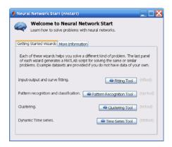
**2** Click **Pattern Recognition Tool** to open the Neural Network Pattern Recognition Tool. (You can also use the command nprtool.)
