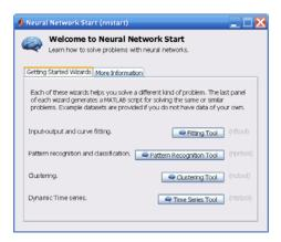
**2** Click **Time Series Tool** to open the Neural Network Time Series Tool. (You can also use the command ntstool.)
