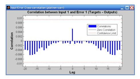
This input-error cross-correlation function illustrates how the errors are correlated with the input sequence x(t). For a perfect prediction model, all of the correlations should be zero. If the input is correlated with the error, then it should be possible to improve the prediction, perhaps by increasing the number of delays in the tapped delay lines. In this case, all of the correlations fall within the confidence bounds around zero.
