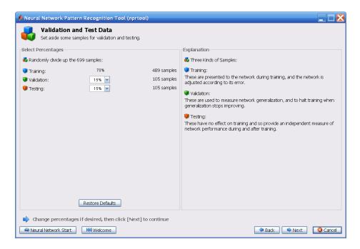
Validation and test data sets are each set to 15% of the original data. With these settings, the input vectors and target vectors will be randomly divided into three sets as follows:
