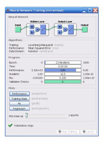
This training stopped when the validation error increased for six iterations, which occurred at iteration 23. If you click **Performance** in the training window, a plot of the training errors, validation errors, and test errors appears, as shown in the following figure. In this example, the result is reasonable because of the following considerations:
