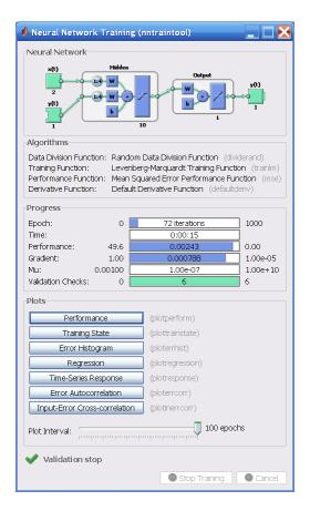
**10** Under **Plots**, click **Error Autocorrelation**. This is used to validate the network performance.
