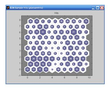
The default topology of the SOM is hexagonal. This figure shows the neuron locations in the topology, and indicates how many of the training data are associated with each of the neurons (cluster centers). The topology is a 10-by-10 grid, so there are 100 neurons. The maximum number of hits associated with any neuron is 22. Thus, there are 22 input vectors in that cluster.
