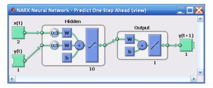
From this figure, you can see that the network is identical to the previous open-loop network, except that one delay has been removed from each of the tapped delay lines. The output of the network is then y(t + 1) instead of y(t). This may sometimes be helpful when a network is deployed for certain applications.
