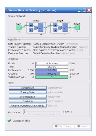
This training stopped when the validation error increased for six iterations, which occurred at iteration 24.
