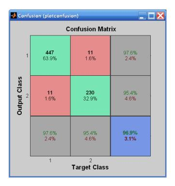
The diagonal cells show the number of cases that were correctly classified, and the off-diagonal cells show the misclassified cases. The blue cell in the bottom right shows the total percent of correctly classified cases (in green) and the total percent of misclassified cases (in red). The results show very good recognition. If you needed even more accurate results, you could try any of the following approaches:
