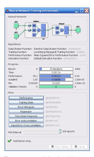
This training stopped when the validation error increased for six iterations, which occurred at iteration 70.
