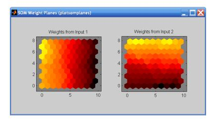
This figure shows a weight plane for each element of the input vector (two, in this case). They are visualizations of the weights that connect each input to each of the neurons. (Darker colors represent larger weights.) If the connection patterns of two inputs were very similar, you can assume that the inputs are highly correlated. In this case, input 1 has connections that are very different than those of input 2.
