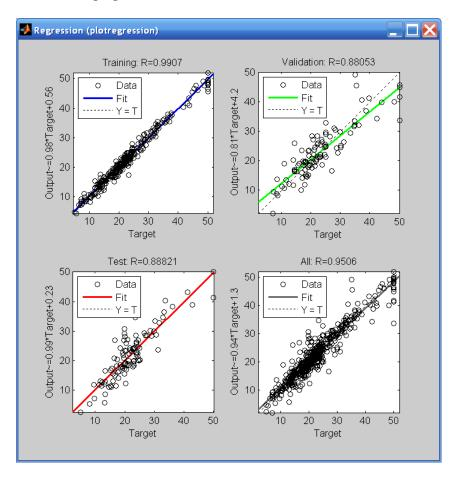
The output tracks the targets very well for training, testing, and validation, and the R-value is over 0.95 for the total response. If even more accurate results were required, you could try any of these approaches:
